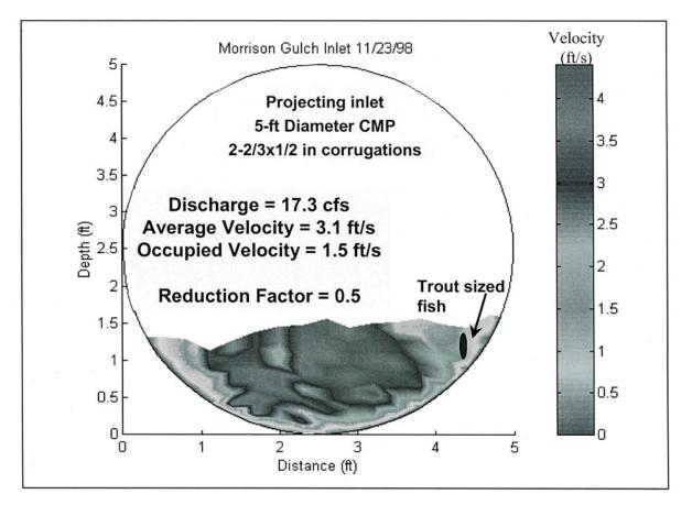
Figure IX- 20. Varying velocity measurements within a culvert on Quarry Road at Morrison Gulch, tributary to Jacoby Creek, Humboldt Bay watershed.
