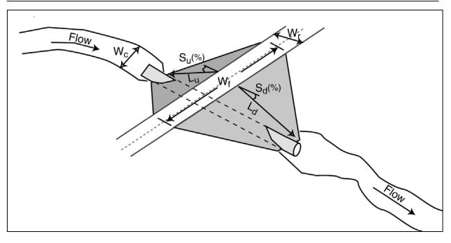
Figure IX- 6. Measurements taken to calculate fill volume.
