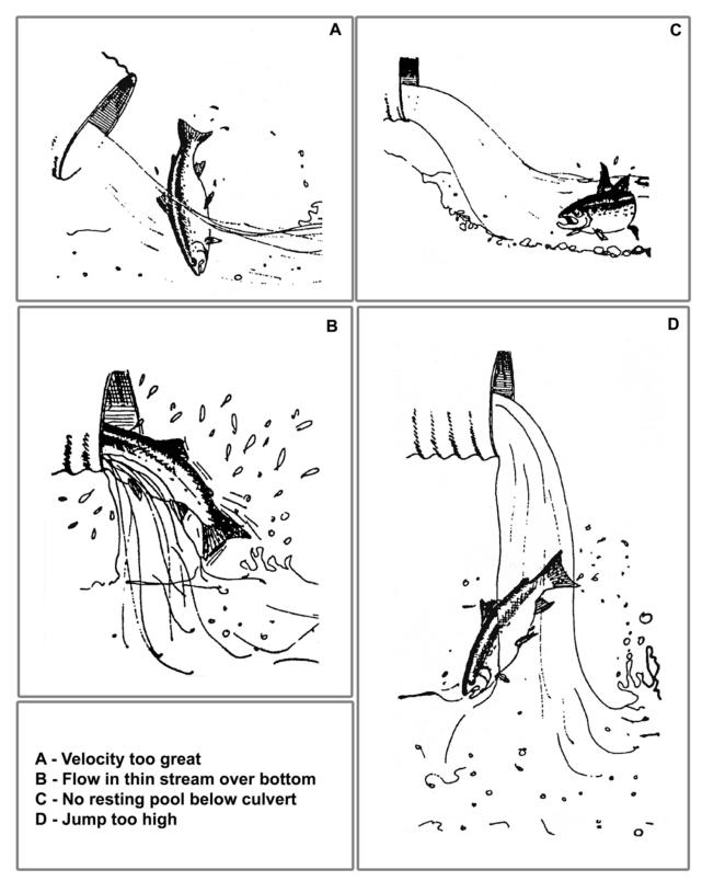
Figure 1: IX Common conditions that block fish passage.
