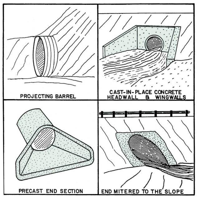
Figure IX- 9. Four standard inlet types (Norman et al. 1985).
