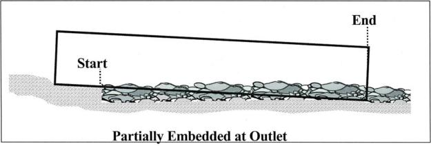
Figure IX- 13. Measurements taken at embedded culverts.
