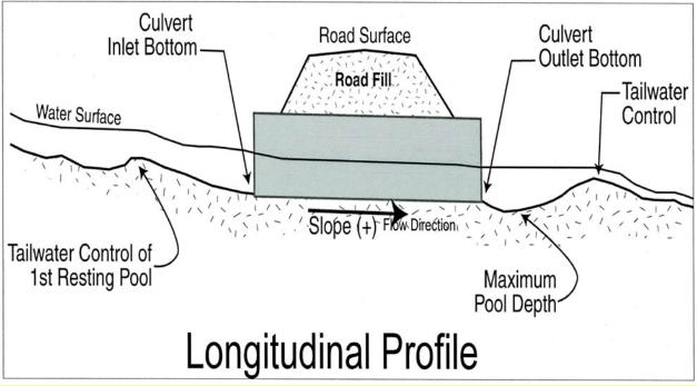
Figure IX- 7. Diagram of required survey points for a longitudinal profile through a culvert.
