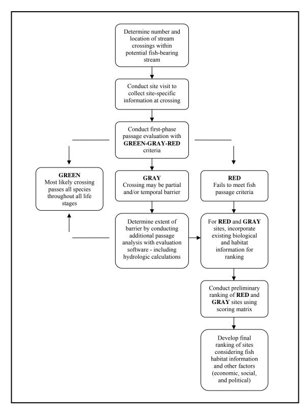
Figure IX- 2. Framework for inventory and evaluation of fish passage through stream crossings.
