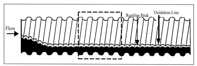
Figure IX- 12. Rustline measurements (Oxidation line is whitish or silver line, not to be confused with the rustline). (Adapted from Flannigan).
