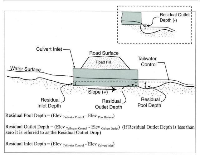
Figure IX- 16. Measurements used in filtering criteria.
