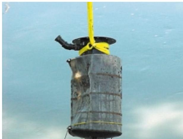
**Figure 14. Butte Creek Farms screen 4/12/99 (screen failure)**
