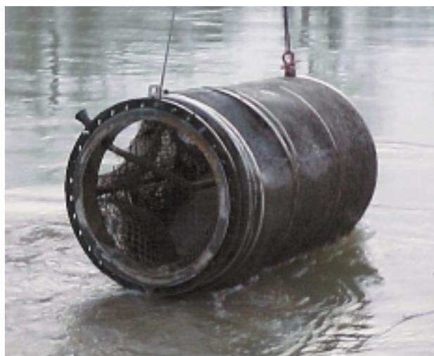
system was ineffective and failed in just a matter of minutes due to the suction load on the screen. Figure 14 shows another screen with a similar clogging failure due to poor cleaning.
