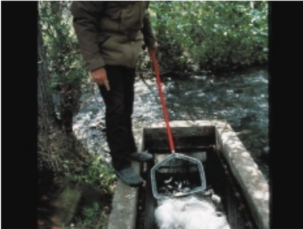
river, we construct a concrete box (Figure 14). Then we periodically put another screen into the box and, as the bypass water from the stream comes into the box, we trap whatever fish are in there. We can then ascertain fish species and obtain an estimate of the numbers of fish that are being saved by the screen.
