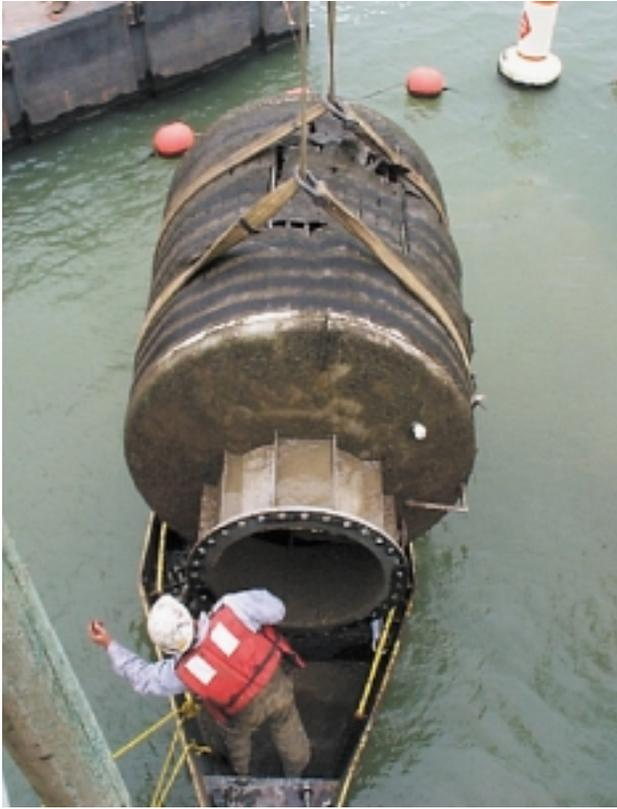
**Figure 16. Corroded screen (inside view)**
